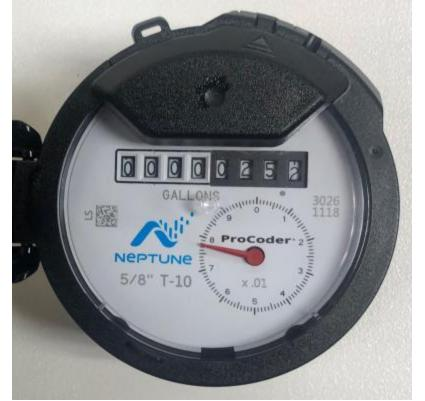
Once the meter box lid has been removed, lift the round cap up from the face of the meter.
